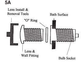
NOTE: Do not twist LED light into socket. Use gentle pressure and push LED light into place.
